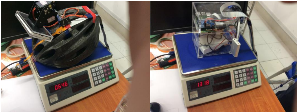
Figure 6.1.1 Weighing the on-head and off-head parts
